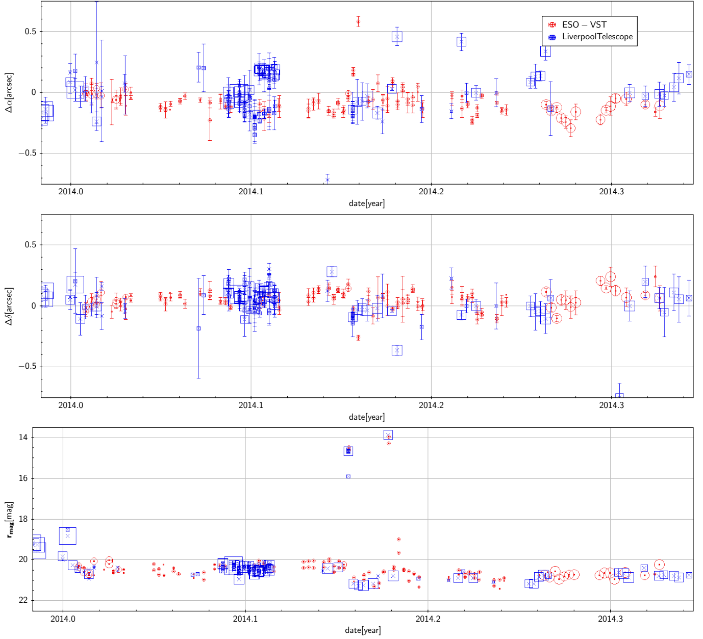
Figure 6. The GBOT measurements since launch. The upper panel shows the O - C residua for the right ascension, the middle panel for declination, and the lower panel the development of the magnitude (mostly r_{\text{SDSS}} ). The red circular symbols (grey in the printed version) denote data taken with the VST, the blue crosses and squares (dark grey in the printed version) LT-data. The errorbars show the scatter of a given sequence, the large symbols (open circles or squares) centred on the small symbols (filled circles or crosses) are scaled according to the number of target measurements (this may or may not be equal to the number of frames, since the target, i.e. Gaia is not always detected on every frame, or a measurement could be rejected for another reason), larger symbols meaning more detections.
